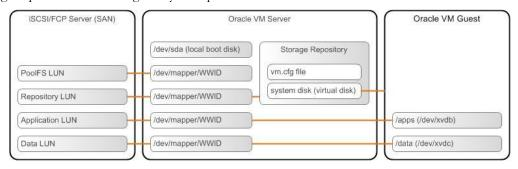
Figure 9: Example Oracle VM deployment architecture showing all storage related objects being presented from SAN servers using block-level protocols such as FCP or iSCSI
