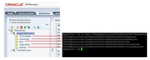
Figure 5: Screen shot showing a storage repository as seen from the perspective of the Oracle VM Manager and Oracle VM Servers
