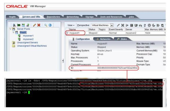
Figure 7: Screen shot showing a specific Oracle VM Guest and the location of the corresponding configuration file on the Oracle VM servers
