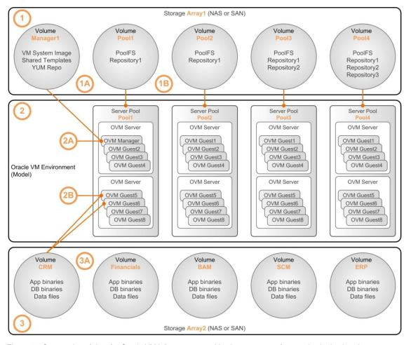
Figure 10: Segregation of data for Oracle VM infrastructure and business systems fosters simpler backup & recovery
